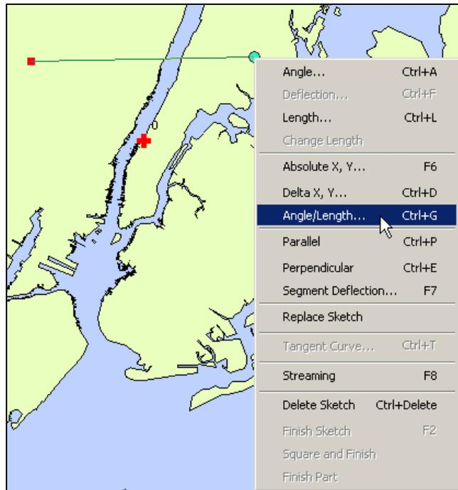
2. The first box is the Angle, the second box in Length. Enter 0 in the Angle box and the number of miles in the Length box. Hit Enter on the keyboard.
